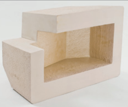
Cast block with removable core and taper of mould
